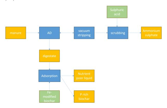
*Figure 7. Cascade 6 – nitrogen recovery and phosphorus recovery on Fe-modified biochar.*
