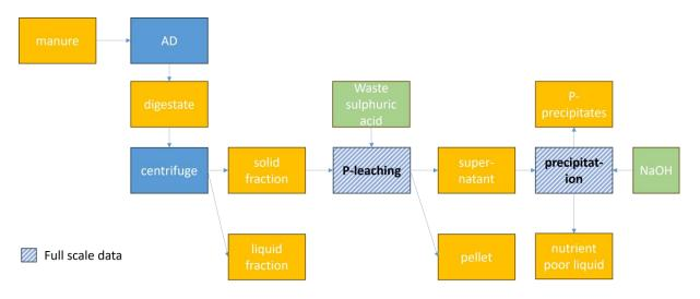
Figure 3. Cascade 2 – phosphorus recovery from pig manure.
