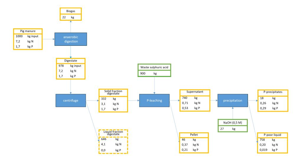
*Figure 11. Cascade 2 - mass and nutrient balance implementing phosphorus recovery from pig manure.*
