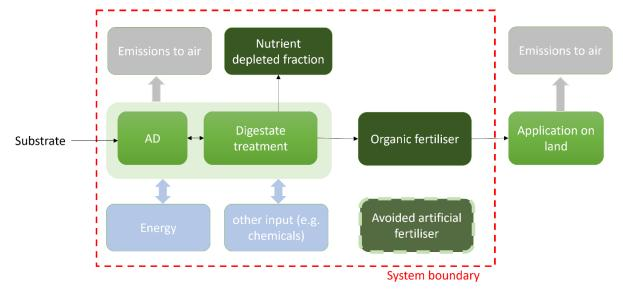
*Figure 17. Generalized scheme of emissions related to the different technology cascades.* The red dashed line represents the system boundary.
