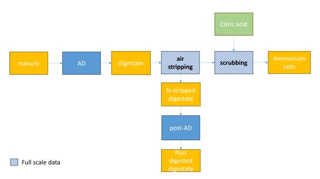
Figure 2. Cascade 1 – post anaerobic digestion and nitrogen recovery from dairy manure.
