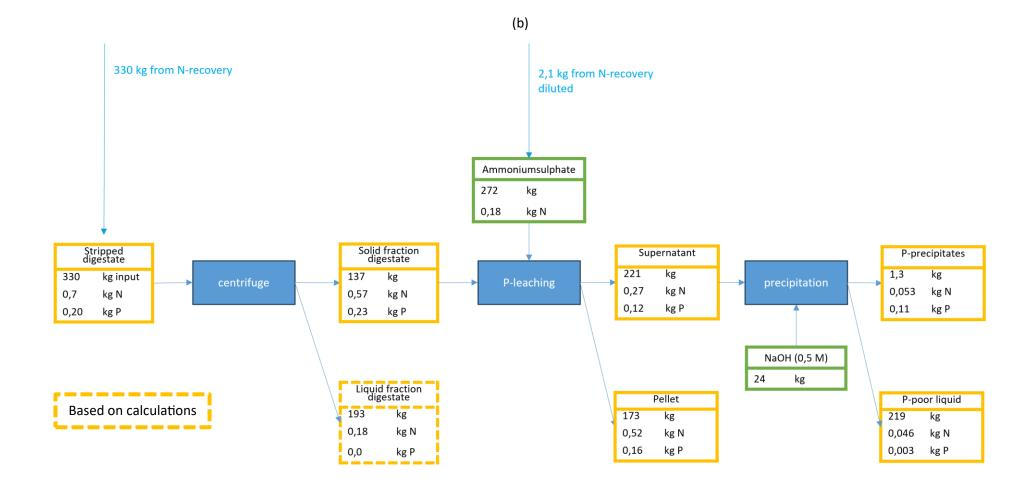
Figure 12. Cascade 3 – mass and nutrient balance implementing (a) post-anaerobic digestion and nitrogen recovery coupled with (b) phosphorus recovery from dairy manure.
