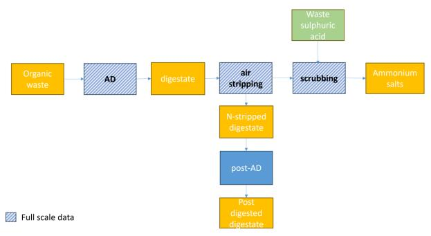
Figure 5. Cascade 4 – post anaerobic digestion and nitrogen recovery from mixed organic waste.
