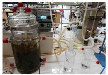
for TAN removal. The effect of lowering pH (from 9.5 to 8) is very limited. The nitrogenrich air stream obtained is typically scrubbed with sulphuric acid. The project sought a safer and more sustainable organic alternative in citric acid and waste sulphuric acid. At lab scale, 91% of the nitrogen present in digestate from cattle manure could be recovered in sulphuric acid (1 M) and 84% in citric acid (60 g/L) with final concentrations of 4,5 g N/kg and 6,2 g N/kg, respectively.
