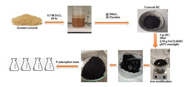
Fe-modified biochar samples were tested in bench-scale batch experiments using synthetic and real digestate samples for phosphate recovery. 50 mL chicken manure digestate with a  $PO_4^{-3}$ -P concentration of 230 mg/L was filled in 100 mL glass flasks without pH adjustment. Flasks were shaken for 90 min.
