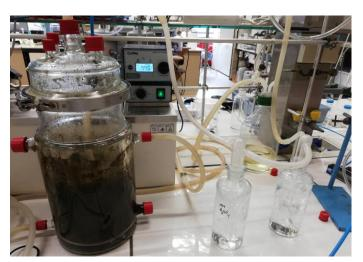
Figure 1: stripping-scrubbing set-up
