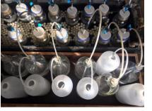
Figure 1: BMP assay set-up, top view
