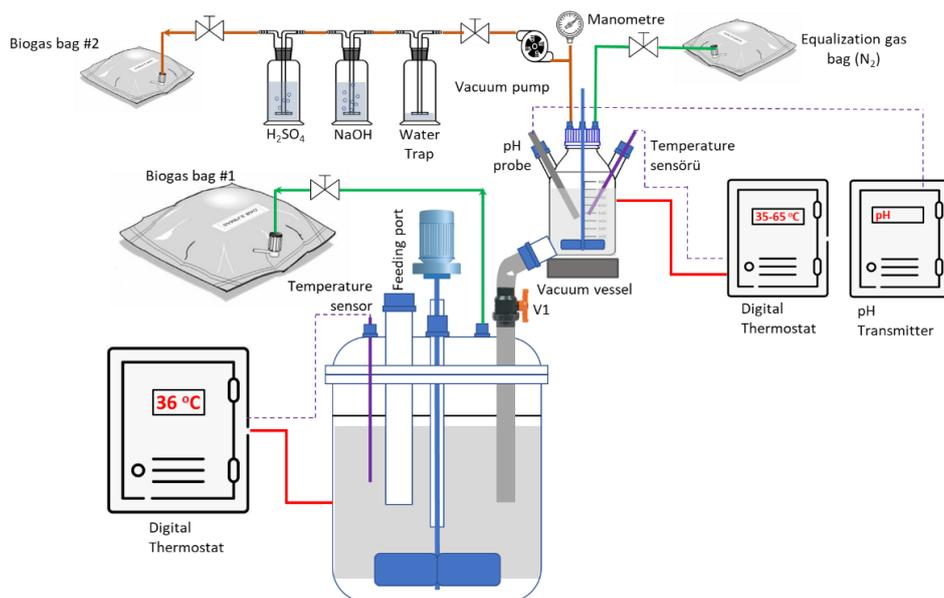
Laboratory scale daily-fed anaerobic reactor integrated with vacuum stripping © Marmara University
